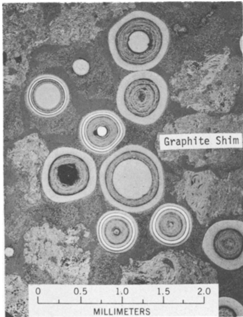
Figure 3 Matrix structure in a thermoplastic pitch-based rod.
